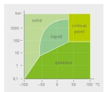
When pressure and temperature exceed the 'critical point' of 74 bar and 31°C, CO<sub>2</sub> combines the benefits of gas and liquid solvents. The properties of the CO<sub>2</sub> as a solvent can be controlled by varying pressure and temperature. This allows you to extract precisely the components you require. The trick is to identify the perfect parameters for each raw material. This process is suitable for almost any kind of dried herb and spice.
